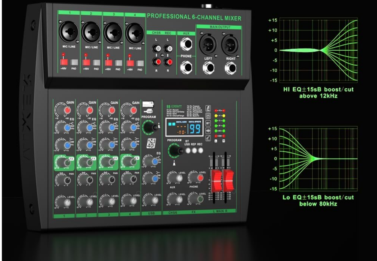
Figure 3.1: High/Low Equalization. This image highlights the High and Low EQ knobs, which allow for balanced tuning to integrate sound more effectively with music.
