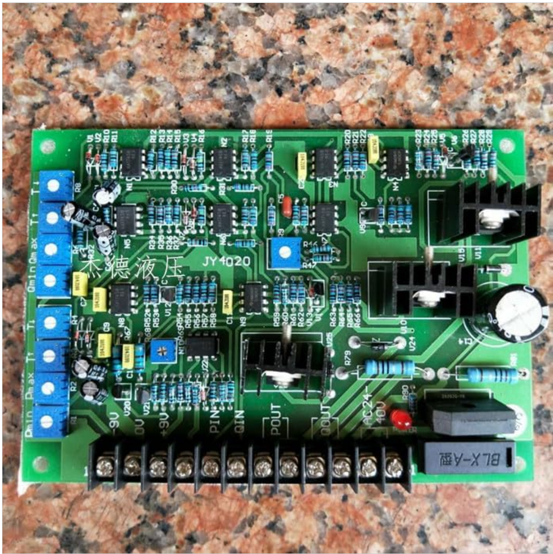
Figure 3.1: Teekos JY4010/JY4020 Double Proportional Valve Amplifier Board. This image displays the main double proportional amplifier board, featuring multiple potentiometers for adjustment, terminal blocks for input/output connections, and various electronic components including integrated circuits and power transistors. The board is green with white silk-screened labels.
