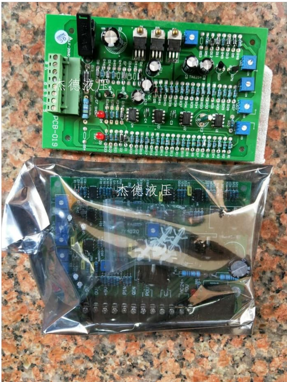
Figure 3.3: Teekos Amplifier Boards. This image displays both the JY4010/JY4020 double proportional amplifier board (partially visible in packaging) and the PCB019 single scale amplifier board, illustrating their relative sizes and packaging.
