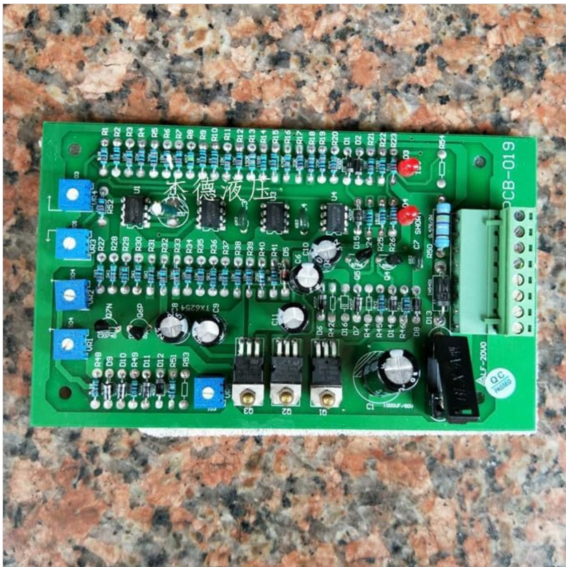
Figure 3.2: Teekos PCB019 Single Scale Amplifier Board. This image shows the single proportional amplifier board, which is smaller than the double proportional board. It also features potentiometers, terminal blocks, and electronic components, designed for single channel proportional control applications.
