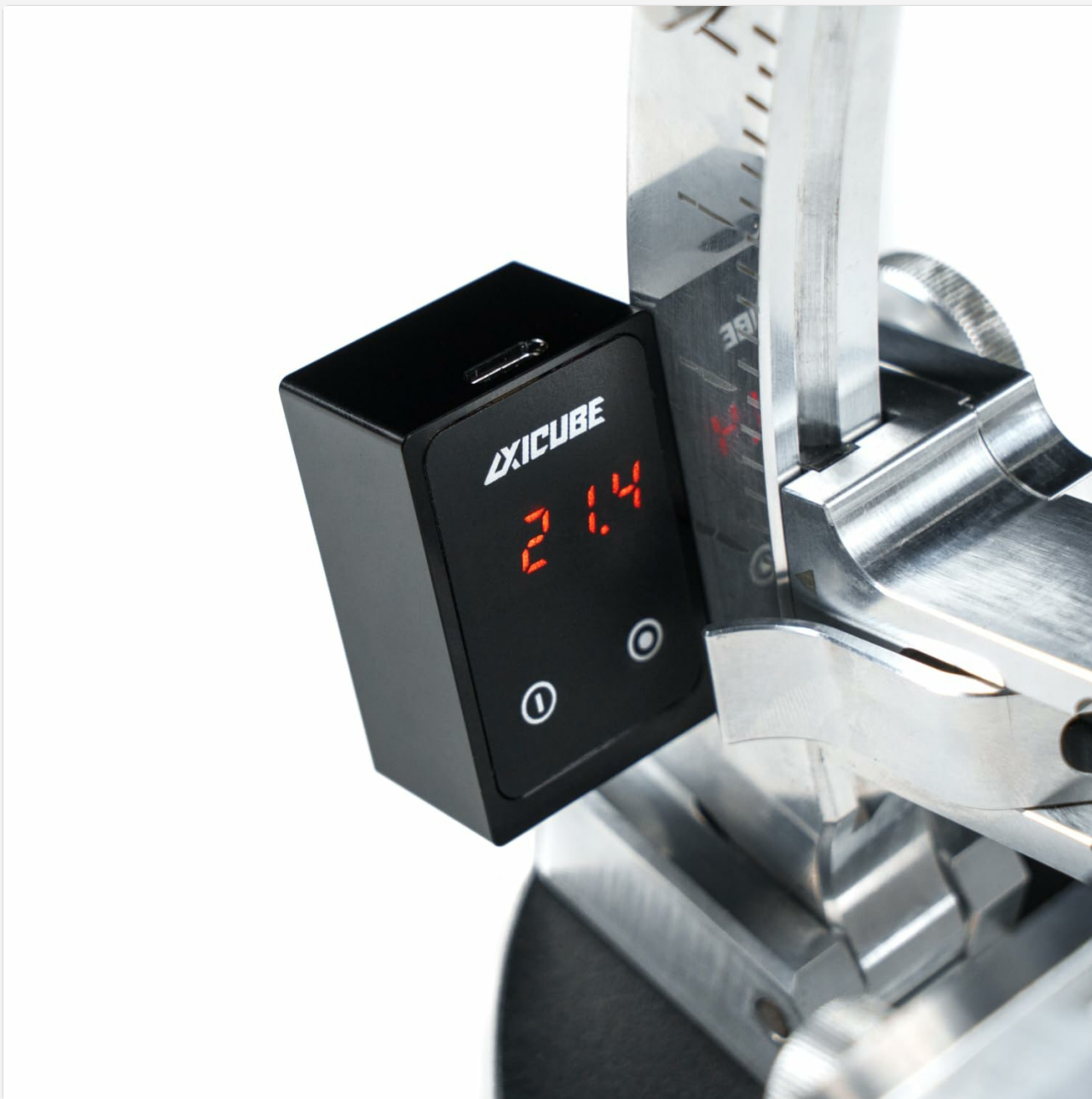
Figure 5.1: Axicube T2 in use, measuring the angle on a sharpening system.
