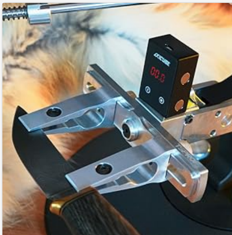
Figure 5.2: Another view of the Axicube T2 measuring an angle on a sharpening setup.
