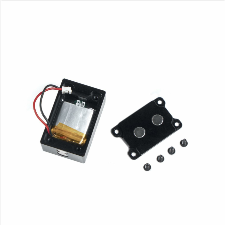
Figure 6.1: Axicube T2 with the battery compartment open, revealing the battery and magnetic cover.
