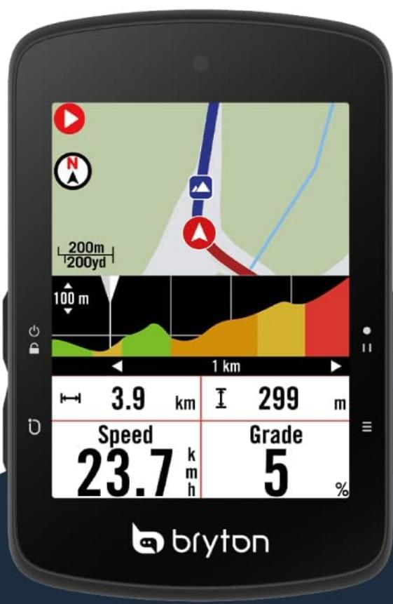
Figure 5: Example of multiple data screens available on the Rider S510.
