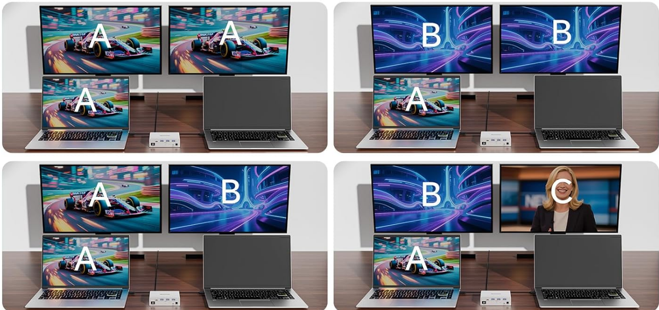
Figure 6: Visual representation of available display modes. This image shows how dual monitors can be configured for Windows (extended and duplicate modes) and macOS (duplicate mode only).
