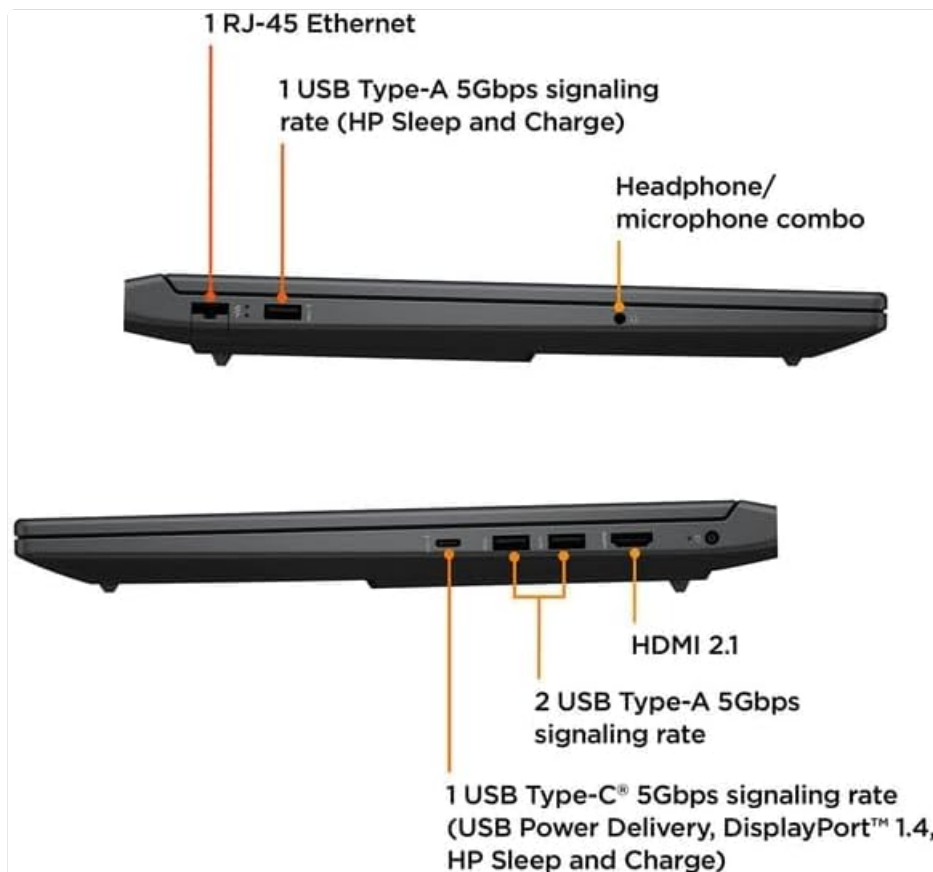
Figure 4.2: Right side ports including HDMI 2.1, two USB Type-A, and one USB Type-C (with Power Delivery and DisplayPort 1.4).
