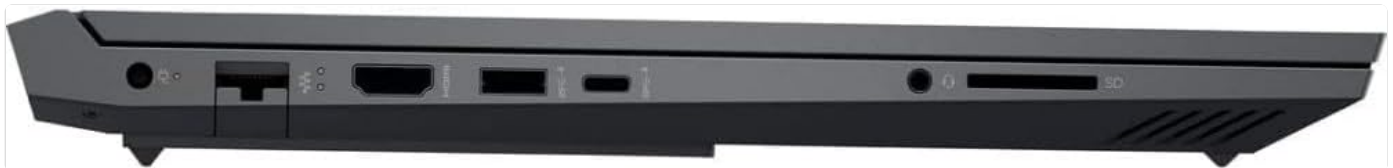
Figure 4.1: Left side ports including RJ-45 Ethernet, USB Type-A, Headphone/Microphone combo, and SD card slot.
