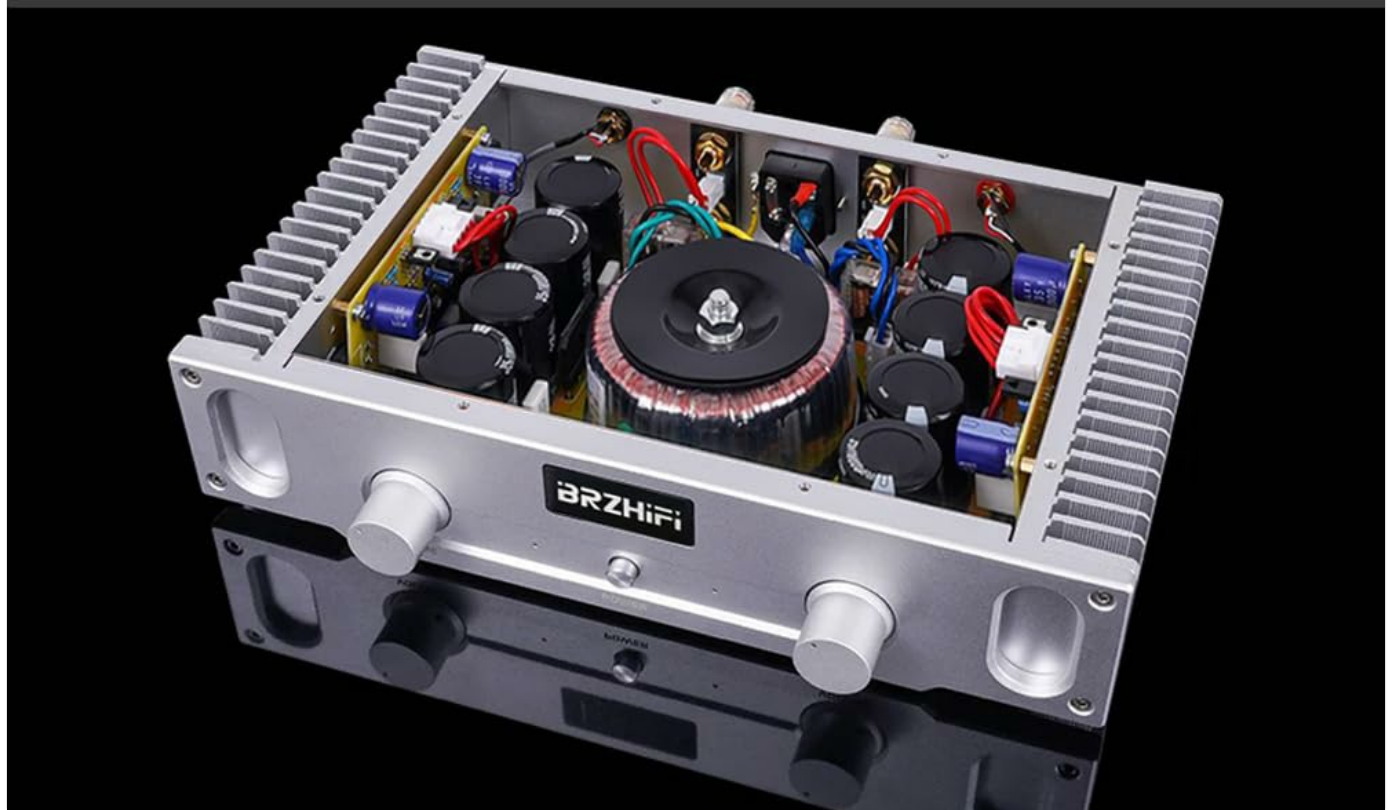
Figure 5: Internal view highlighting the large toroidal transformer.
