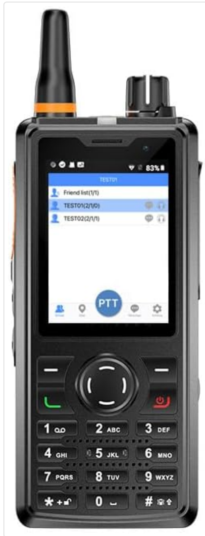
Figure 3: Front view of the ANYSECU T60 radio, displaying the screen with a contact list, the PTT button, and the numeric keypad. The antenna is visible at the top.
