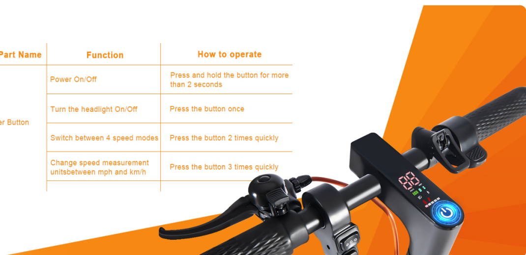
Figure 5: Detailed table outlining the functions of the multi-function button for power, headlights, speed modes, and unit changes.
