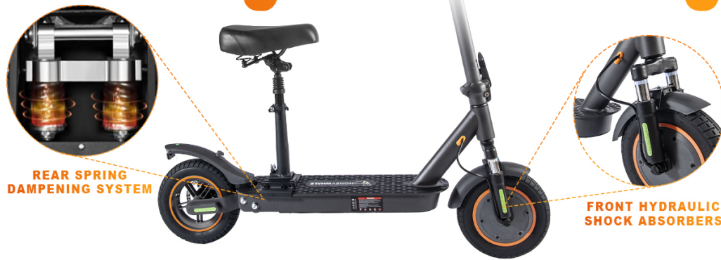
Figure 17: Illustration of the scooter's dual suspension system, featuring both rear spring dampening and front hydraulic shock absorbers.
