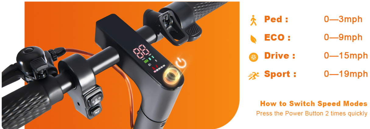
Figure 6: Illustration of the four available speed modes and instructions for switching between them.
