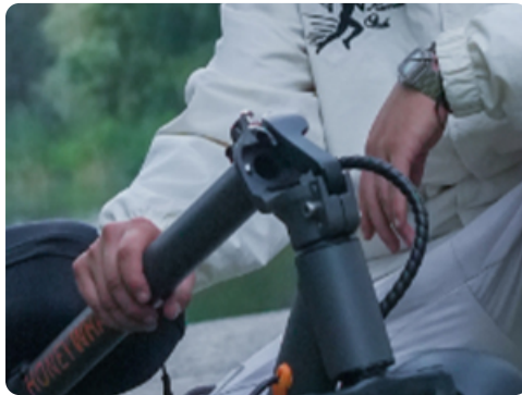
Figure 19: The folding locking ring ensures the handlebar is securely in place during operation.
