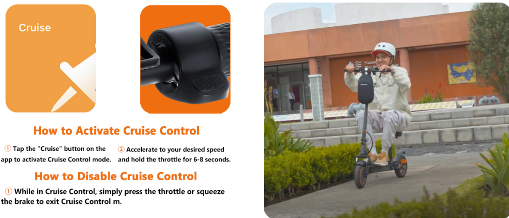
Figure 7: Step-by-step guide on how to activate and deactivate the cruise control feature for a more relaxed ride.
