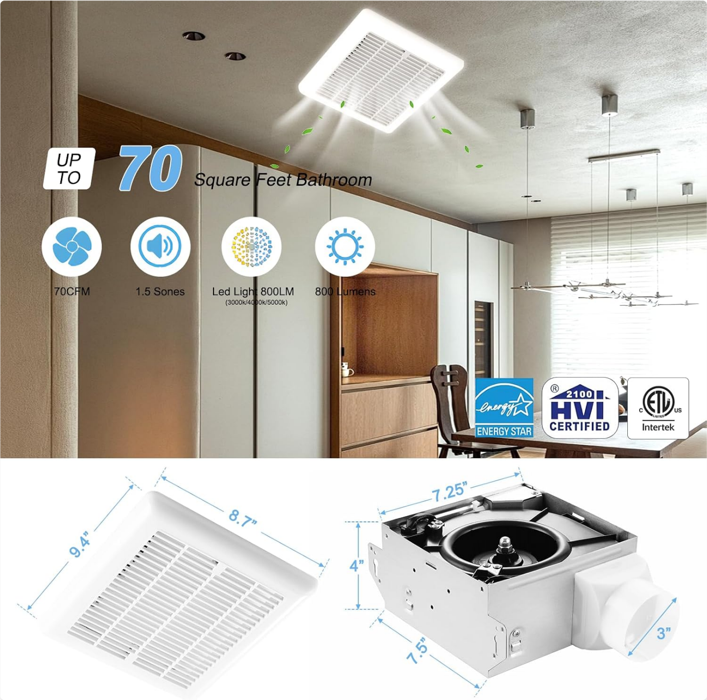
Image: Detailed dimensions of the fan unit and grille, highlighting its certifications.
