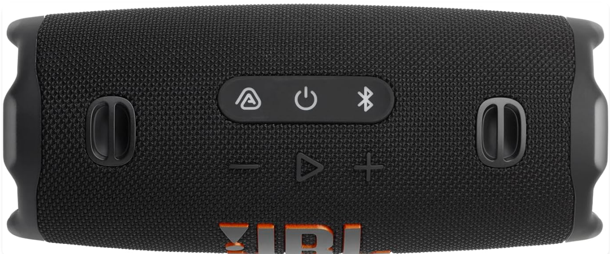
Figure 4: Top panel showing power, Bluetooth, and Auracast buttons.
