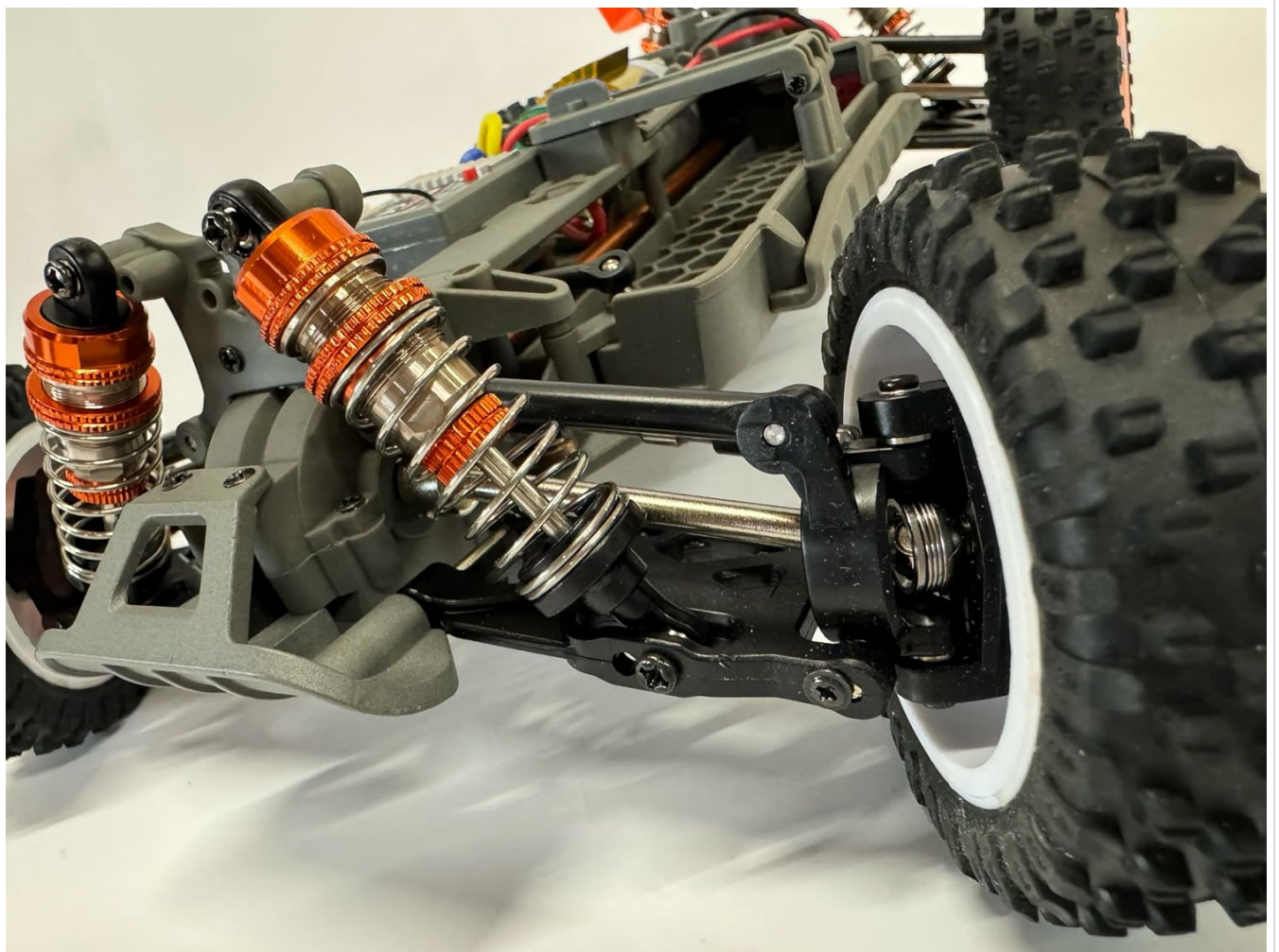
Image: Close-up of the rear suspension, showing the aluminum oil-filled shock absorbers and metal components.
