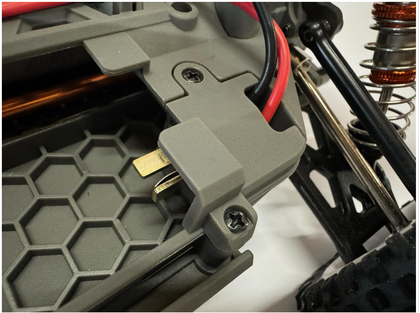
Image: Detail of the battery connector on the vehicle's chassis.
