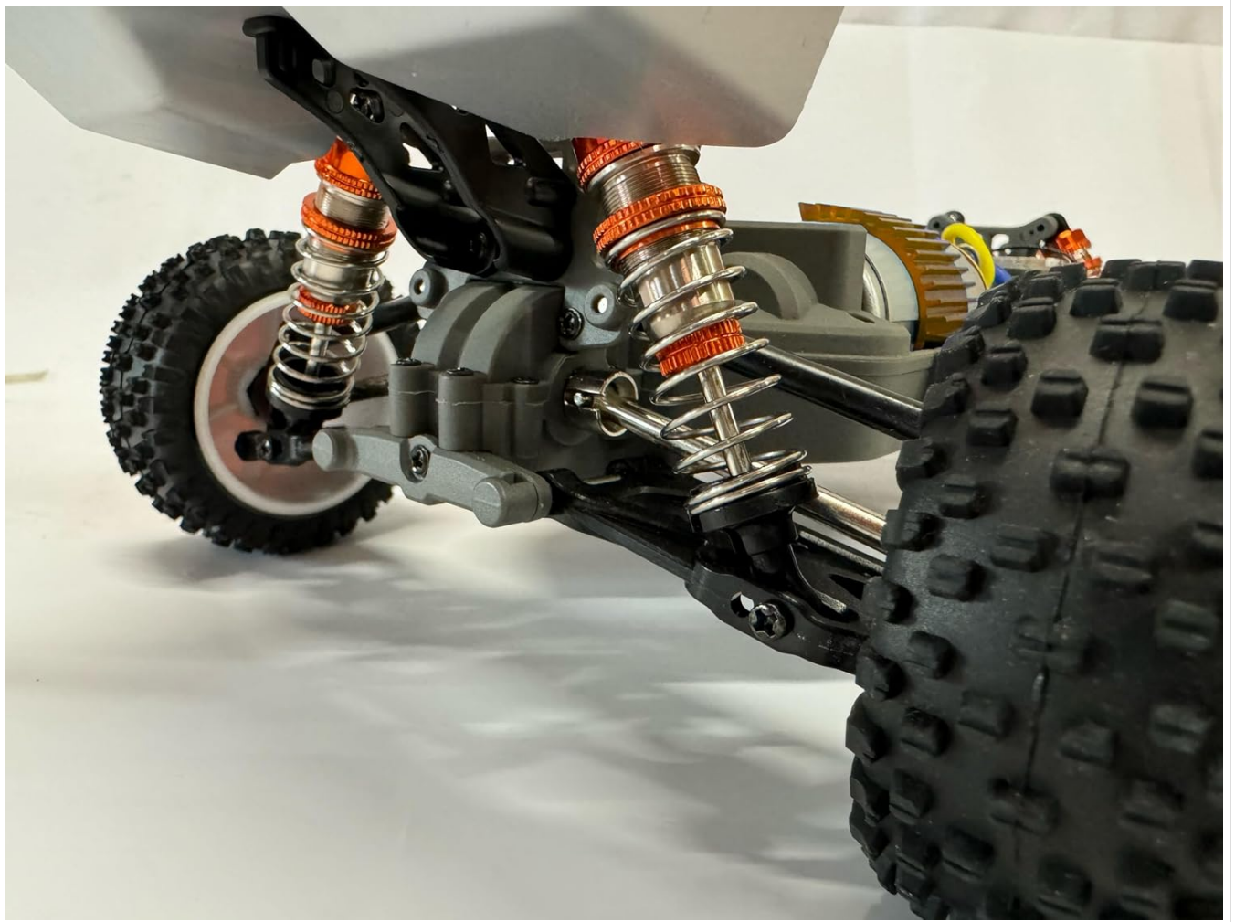
Image: Close-up of the rear suspension, showing the aluminum oil-filled shock absorbers and metal components.
