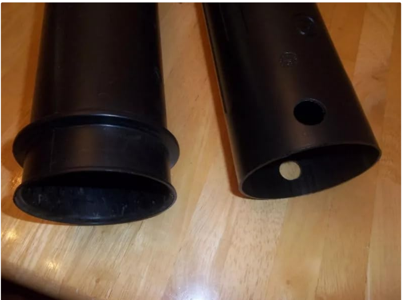
Figure 3: Detailed view of the ends of the blower tubes, illustrating the connection points for secure attachment.
