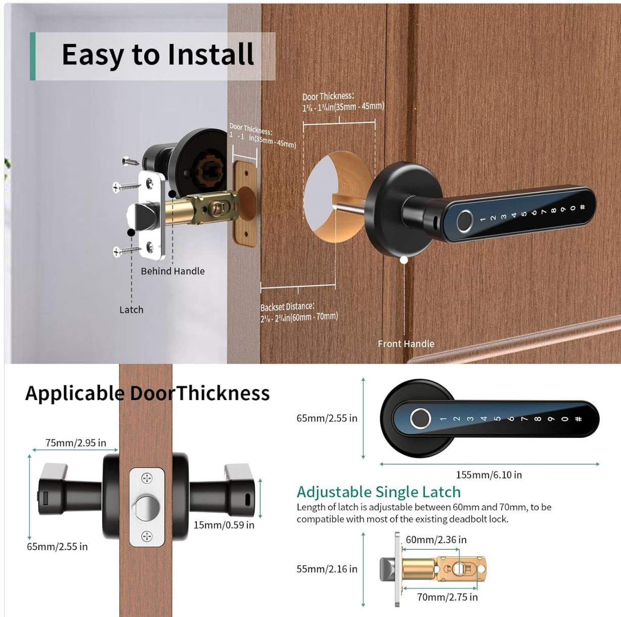
Image 4.1: Detailed installation guide and applicable door dimensions for the smart lock.
