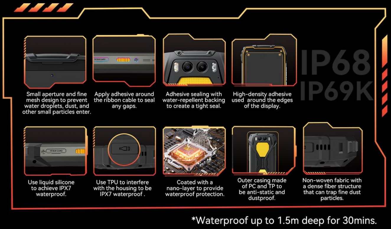
Figure 2.1: Illustration of the SIM/TF card slot and various waterproof sealing points on the Blackview BV7300.
