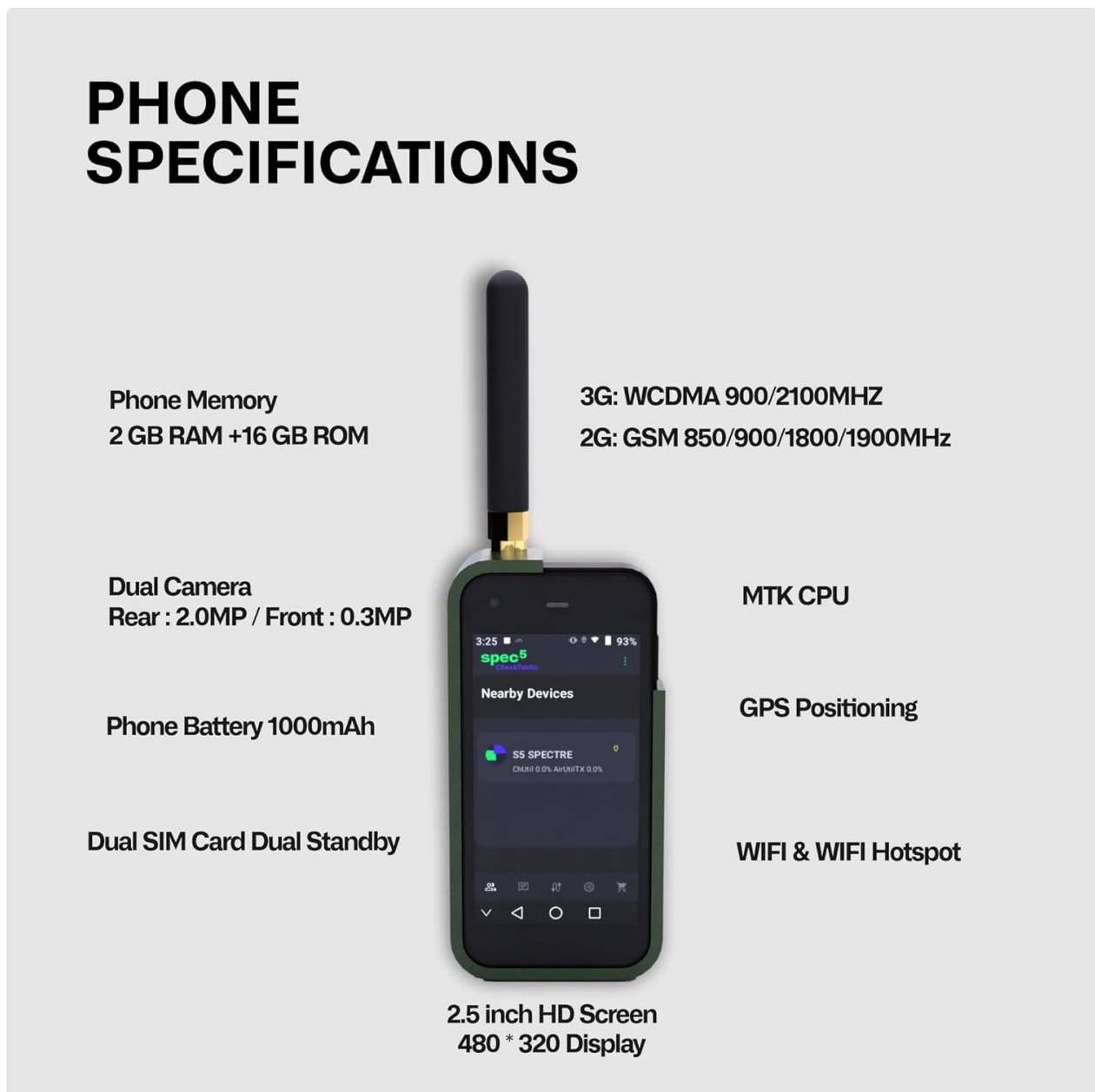
Image 7.2: Specific details regarding the phone's CPU, memory, display, and network capabilities.
