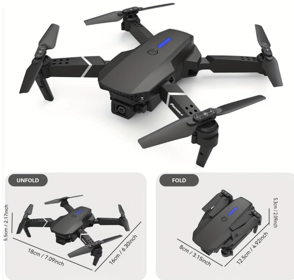
Image: Visual representation of the E88 Drone in its unfolded and folded states, showing its compact design.
