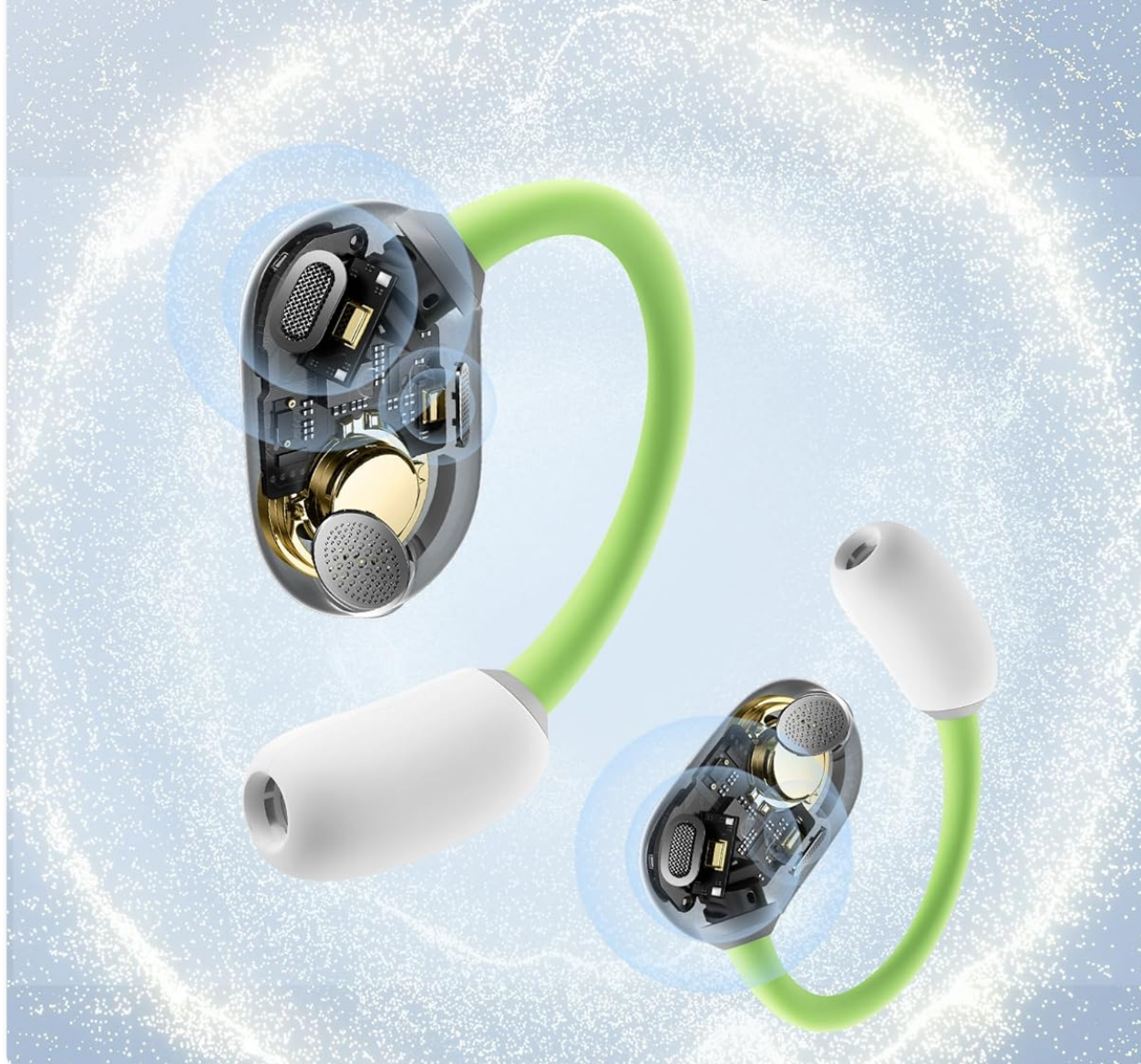
Image: An X-ray view of the earbud's internal components, specifically highlighting the four ENC microphones and their role in enhancing call clarity.
