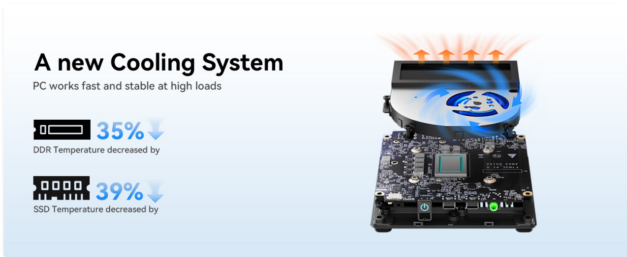
Figure 6: Diagram illustrating the internal cooling system of the KODLIX AD69 Mini PC, showing airflow and heat dissipation components.
