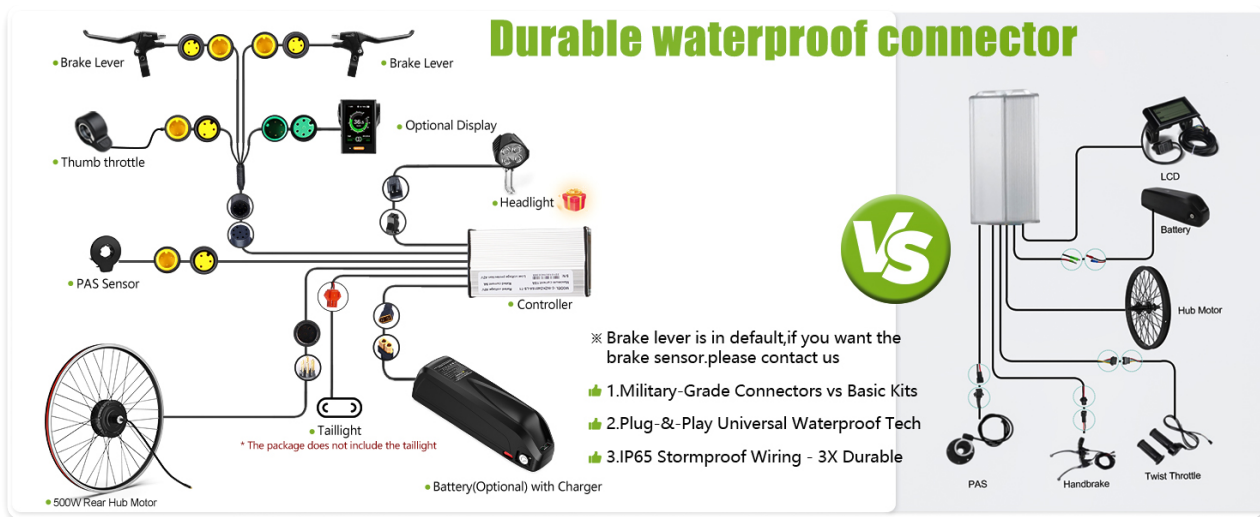
Image: Detailed wiring diagram for the 750W BAFANG Rear Hub Motor kit, showing connections for throttle, brake levers, display, PAS sensor, battery, headlight, and taillight.
