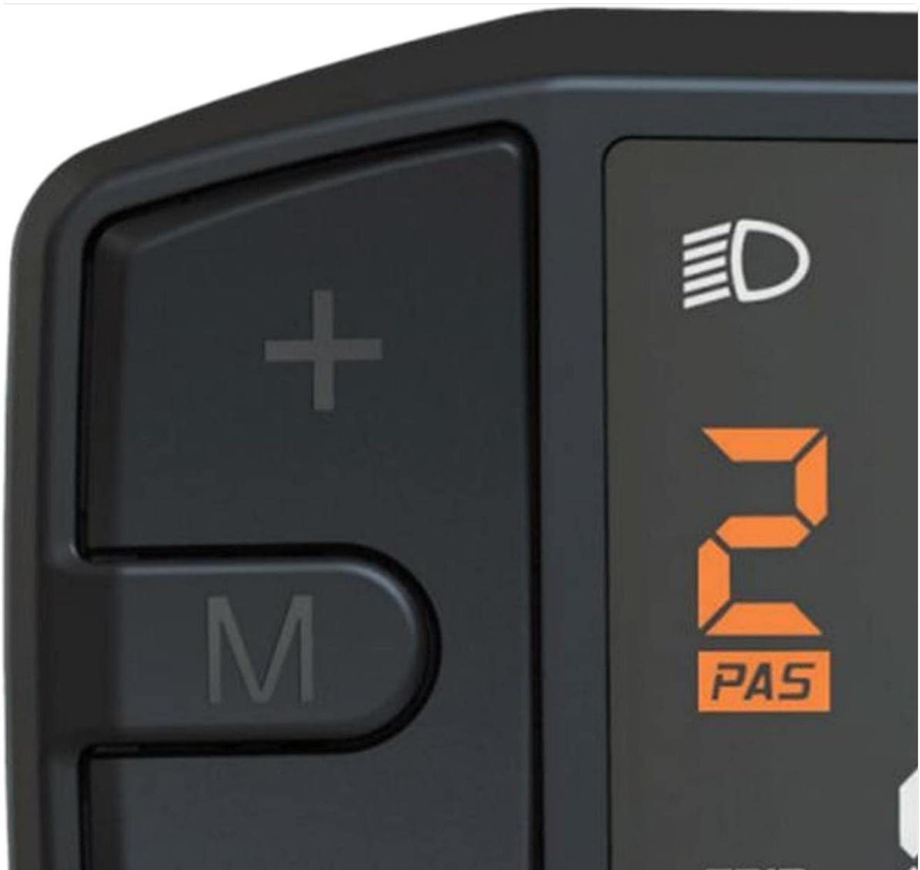
Figure 3.1: Close-up view of the control buttons on the DZ41-CAN display. The image clearly shows the '+', 'M', and '-' buttons, which are used for navigating menus, adjusting settings, and controlling various functions of the e-bike.
