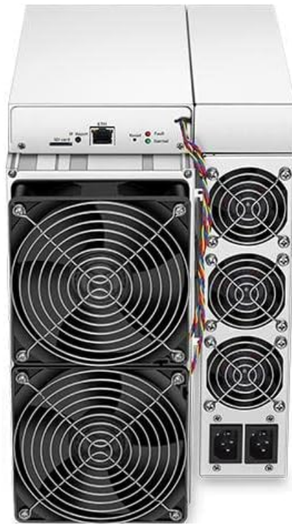
Image 4.1: Rear view of the Antminer L7, illustrating the power input ports and the arrangement of the cooling fans.
