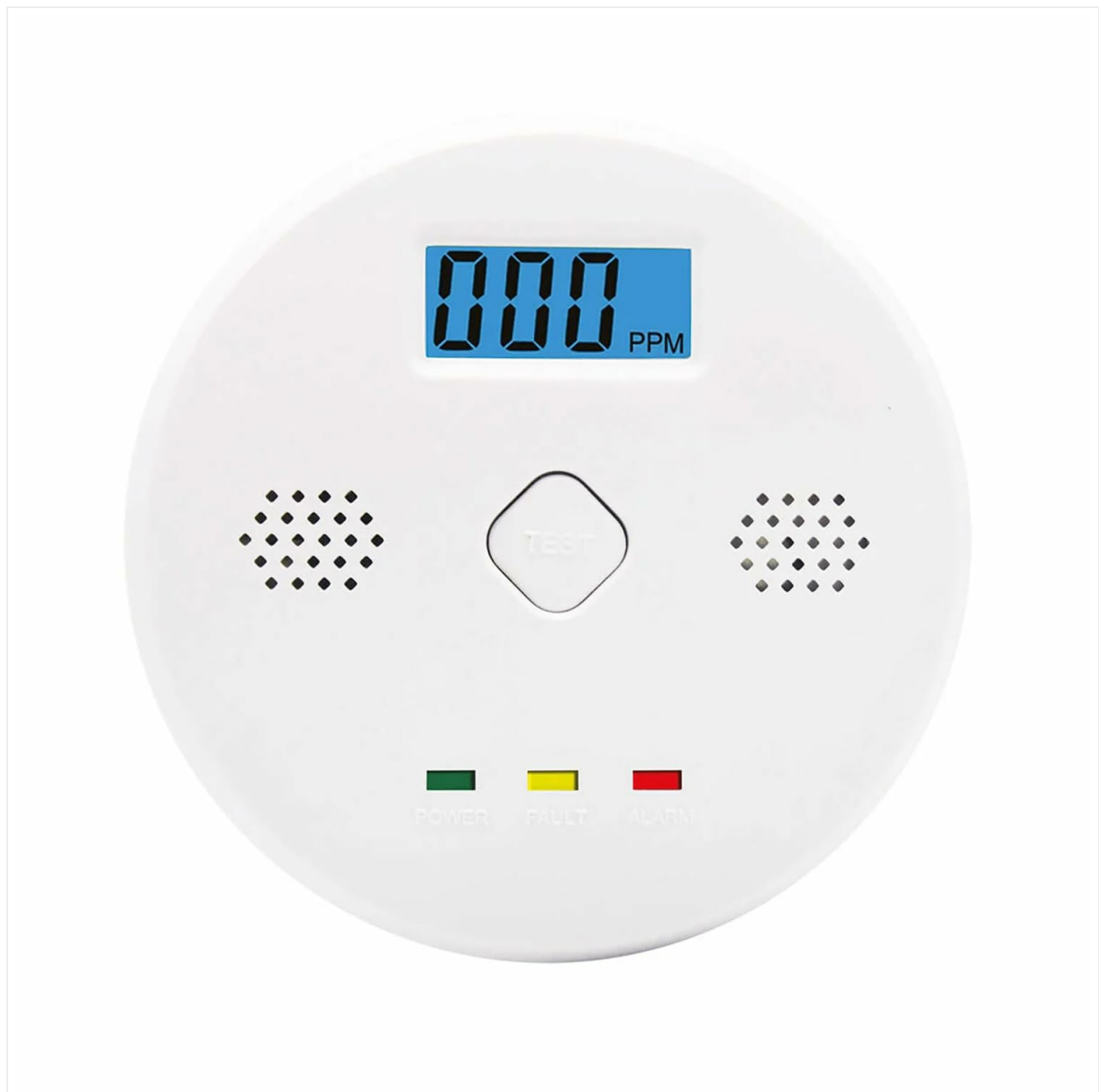
Figure 1: Front view of the GBC iSnatch Carbon Monoxide Detector. It features a central digital display showing PPM (parts per million) of CO, a 'TEST' button, and three indicator lights at the bottom: 'POWER' (green), 'FAULT' (yellow), and 'ALARM' (red). Speaker grilles are visible on both sides of the display.
