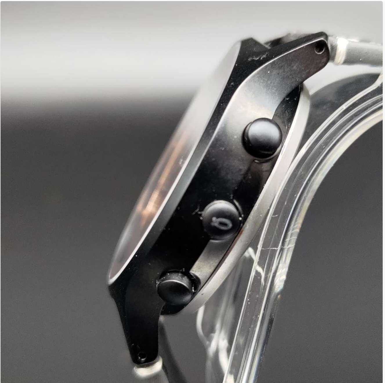
Figure 4.3: Close-up side view of the smartwatch, showing the three distinct black buttons used for various functions and navigation.
