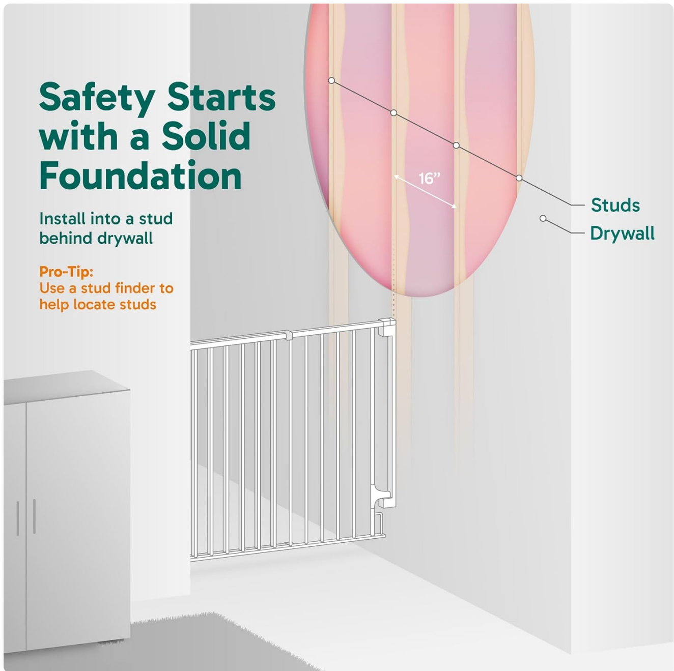
Figure 2.1: Importance of installing into a wall stud for secure mounting.
