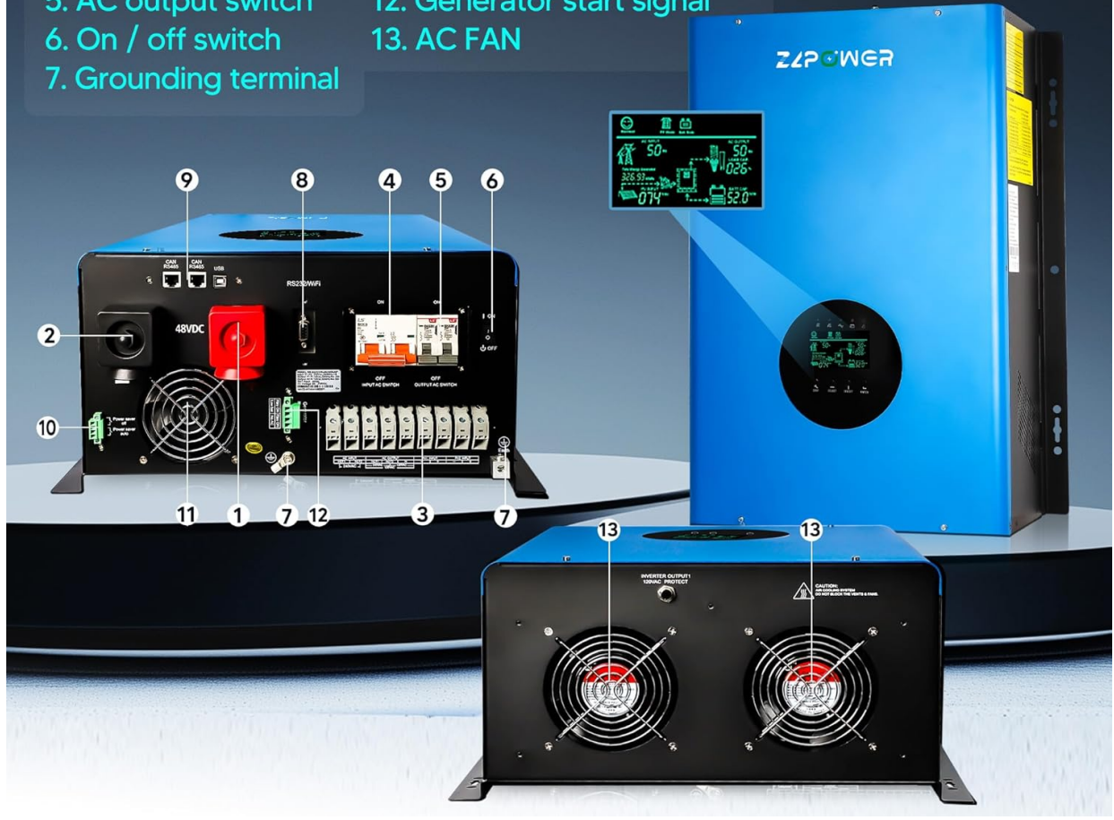
Figure 3.7: Detailed view of the inverter's wiring terminals, including Battery Positive/Negative, Terminal block, AC input/output switch, Grounding terminal, RS-232, CAN/RS485/USB ports, Remote switch, and DC/AC FAN connections.
