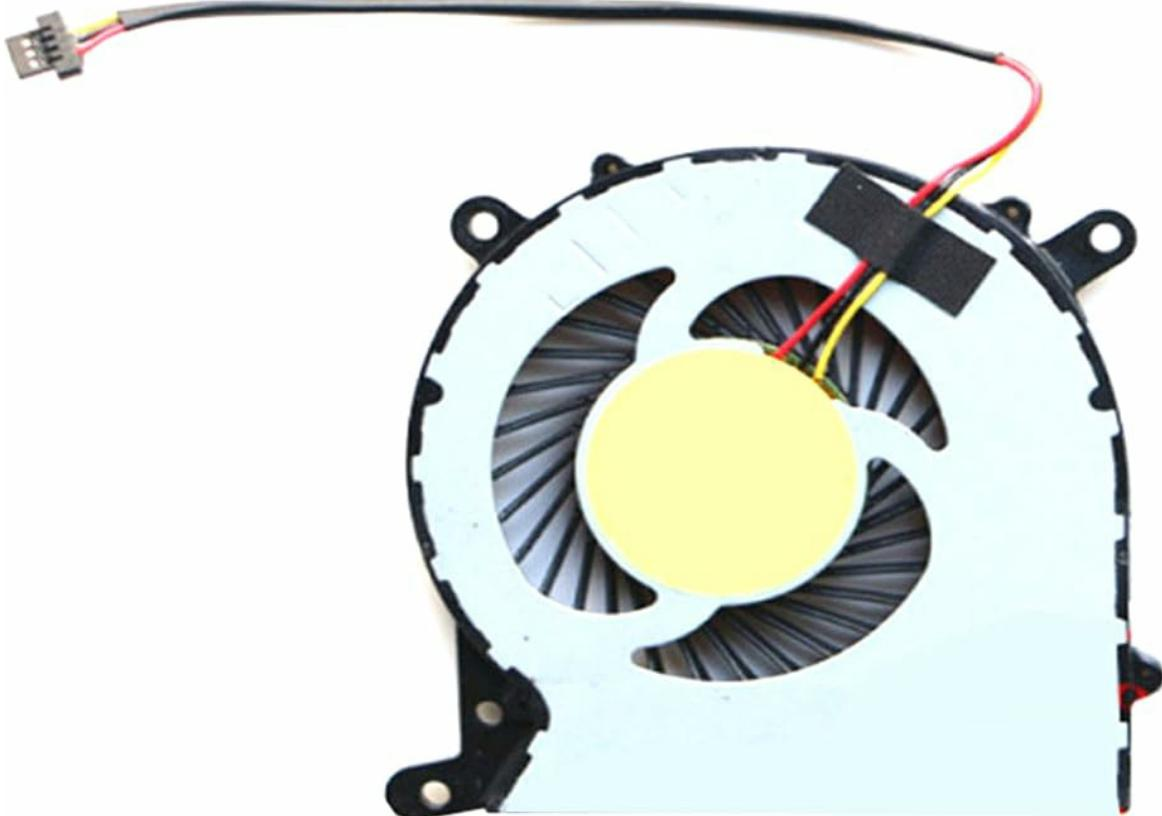
Image: The Generic Laptop CPU Fan, showing its compact design and 3-pin connector. This fan is a critical component for maintaining optimal laptop operating temperatures.
