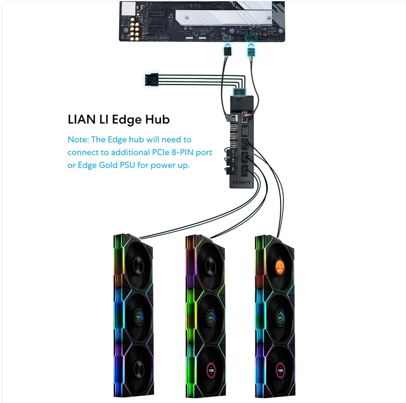
Image: Diagram showing the Lian Li Edge Hub connection for multiple fans.
