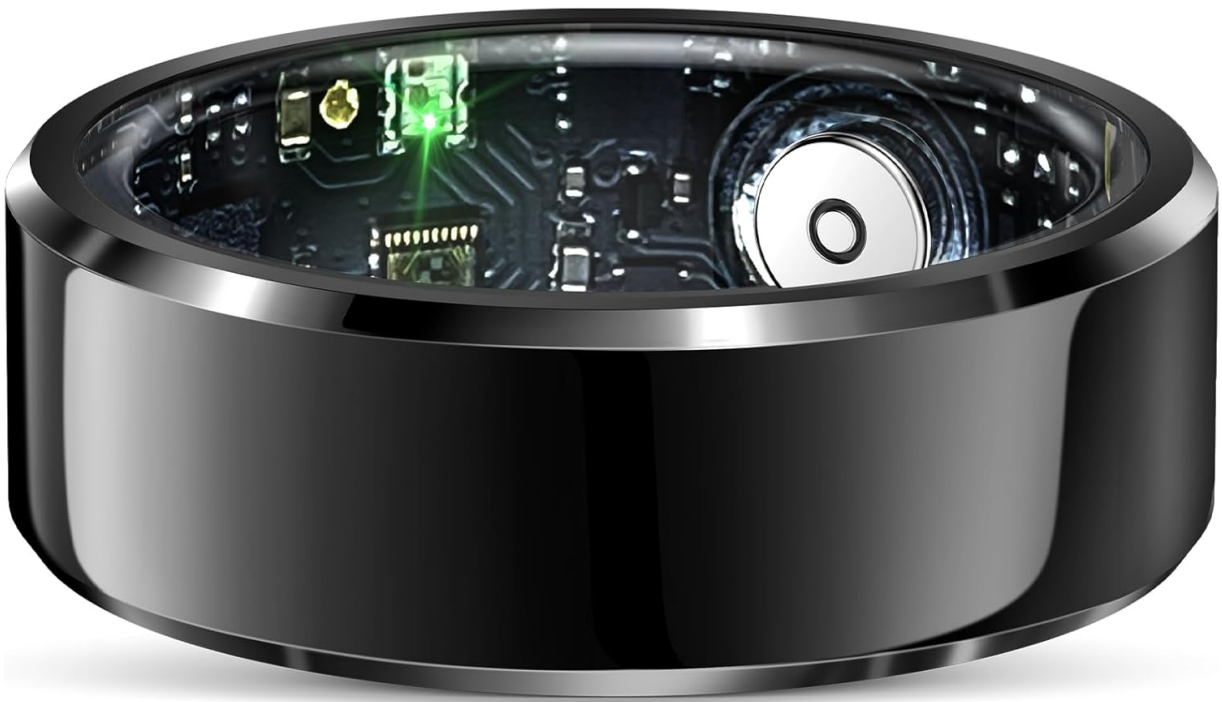
Image 3.1: Detailed view of the Smart Ring R3's interior, showing the optical sensor and circuitry.
