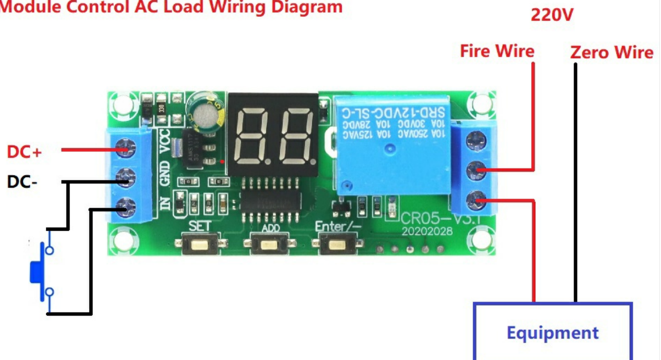
Figure 5.2: Wiring diagram for controlling an AC load. The module is powered by DC 12V (DC+ to VCC, DC- to GND). The trigger
