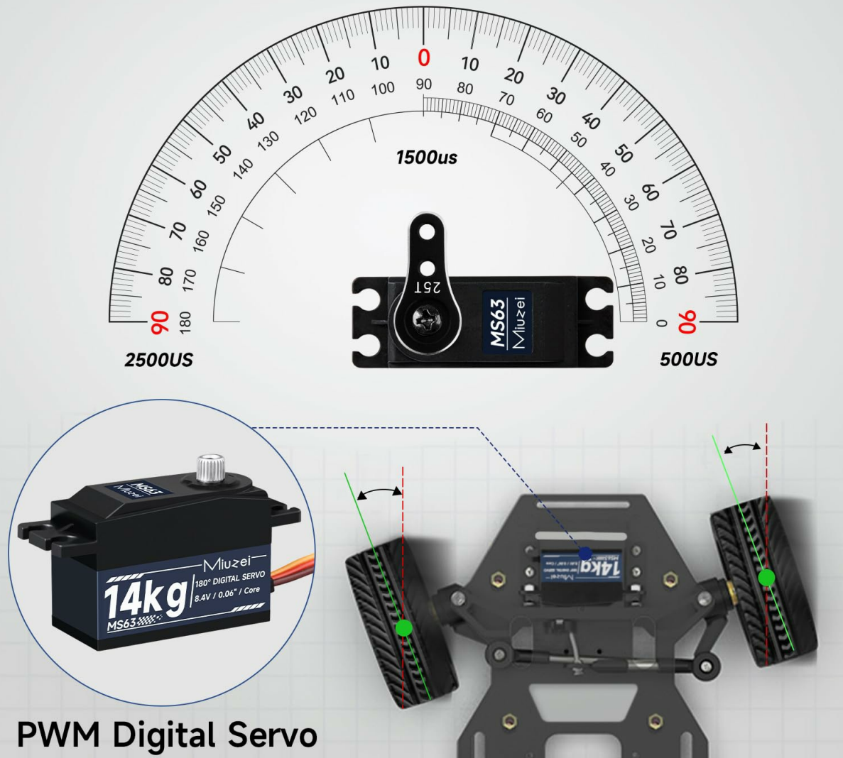
Image 6.1: Quick response and high precision diagram. This image visually explains the servo's angular movement and responsiveness.
