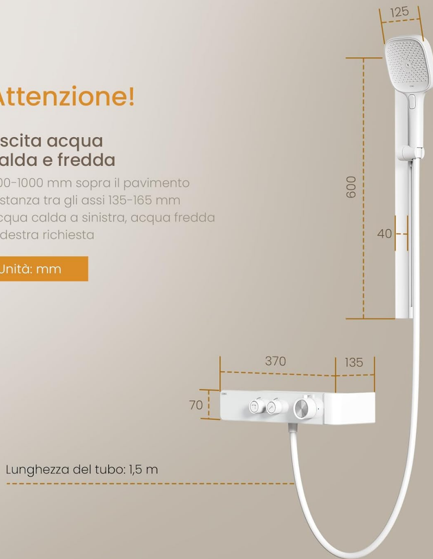
Figure 2.1: Hot and cold water connection requirements and dimensions (Unit: mm). Hot water must be on the left, cold water on the right. The hose length is 1.5 meters.
