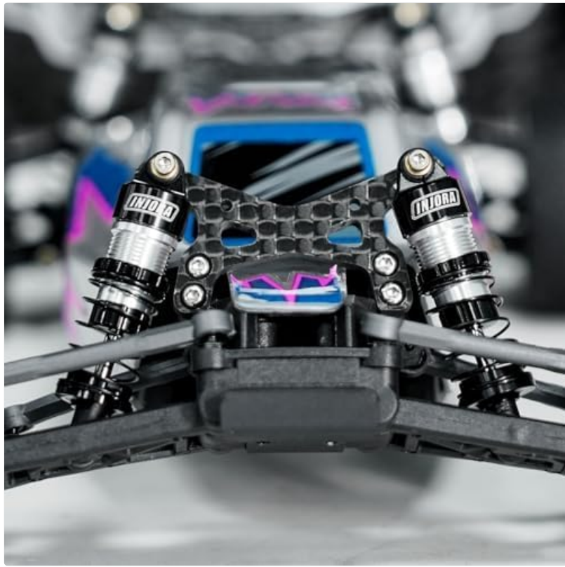
Figure 4: Shocks Installed on RC Buggy
