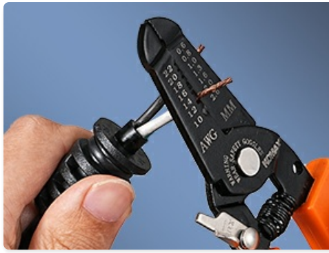
Image 4.1: A hand using a wire stripper to prepare the end of a cable for connection to the GFCI plug.
