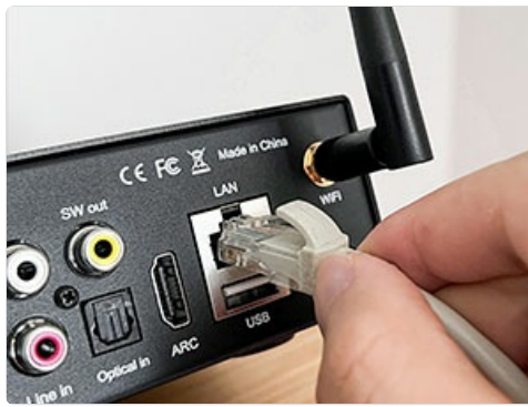
Figure 5: Connecting the H50 to a wired network via the LAN port.
