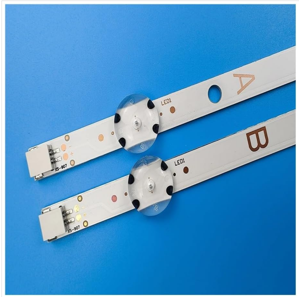
Close-up view of two individual LED backlight strips, showing the LED lenses and connection points. Note the 'A' and 'B' markings for orientation.
