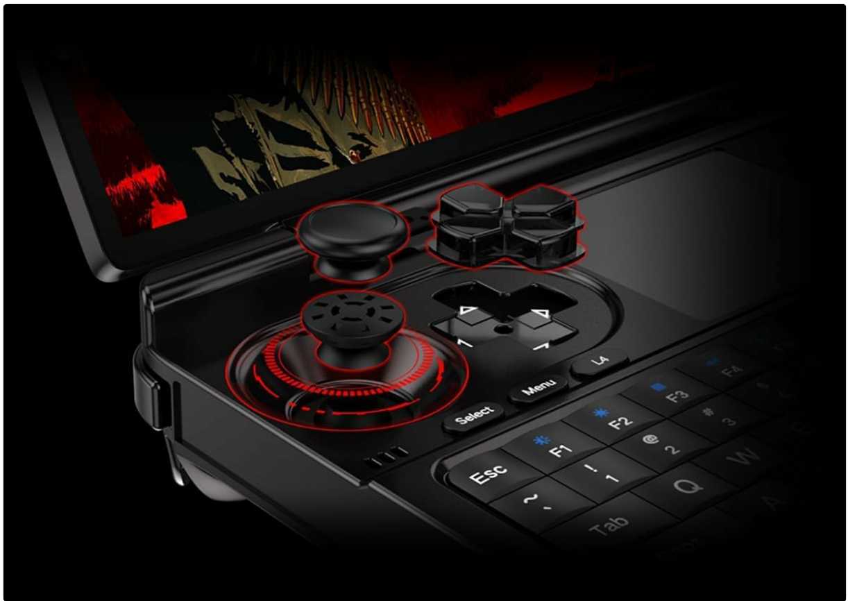
Figure 3.2: Close-up view of the left-side gamepad controls, including the Hall effect joystick and directional pad.
