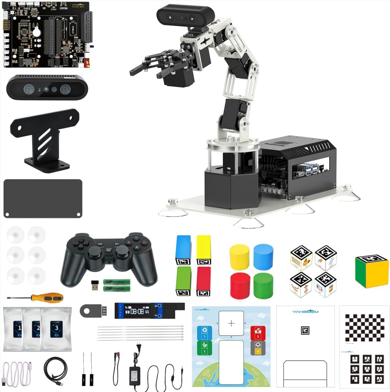
Image: An overview of the Yahboom DOFBOT PRO robotic arm kit, showcasing the main robotic arm assembly, depth camera, control board, and various accessories.
