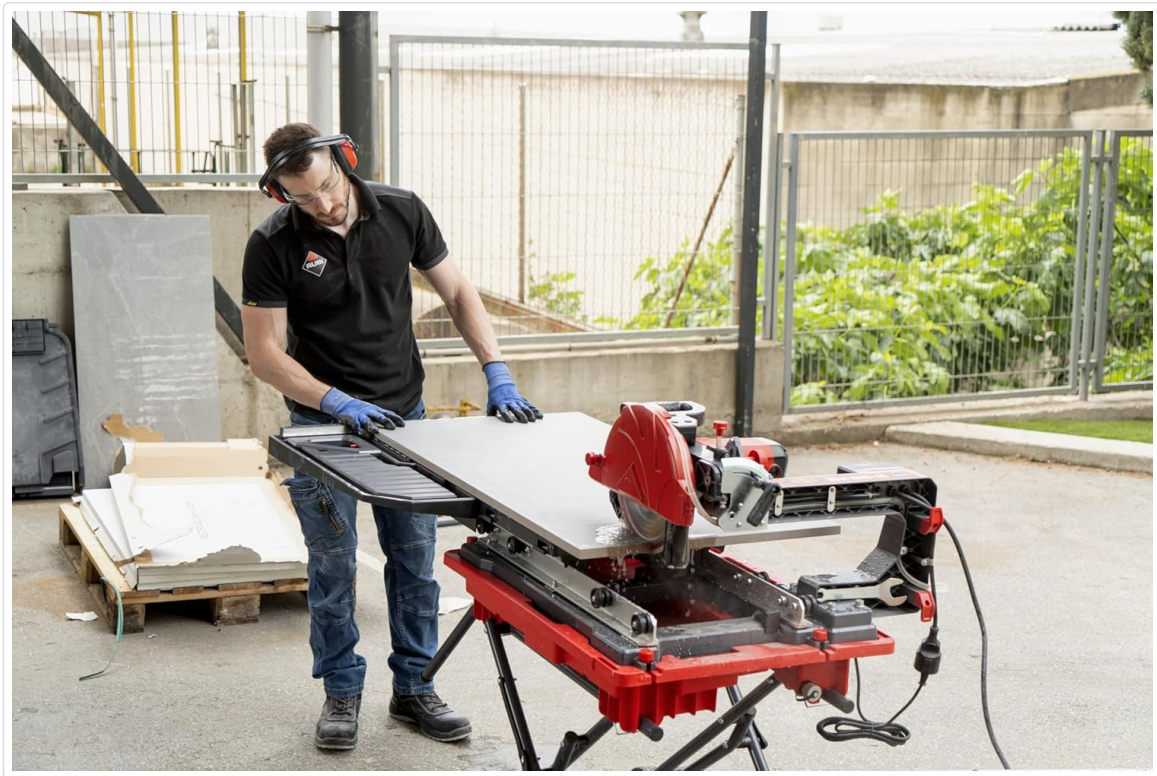
Image 5.1.1: Positioning a large tile for cutting.
