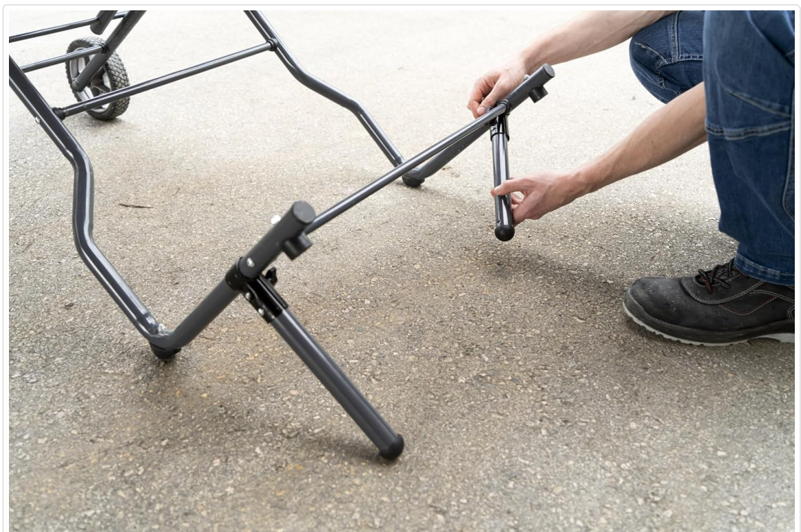
Image 4.2.2: Securing the stability legs to the saw stand.
