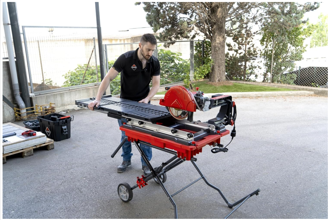
Image 4.1.2: Proper alignment of the extension table during installation.
