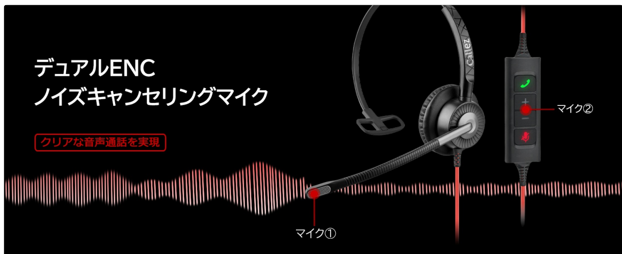
Figure 4.1: In-line Control Unit. This image details the call answer/end/cancel button, volume up/down buttons, and microphone mute button.
