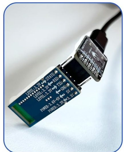
Image 3.1: Contents of the DX-BT24-SET Developer Package, showing the BT24 module, a USB to TTL adapter board, and a USB cable.
