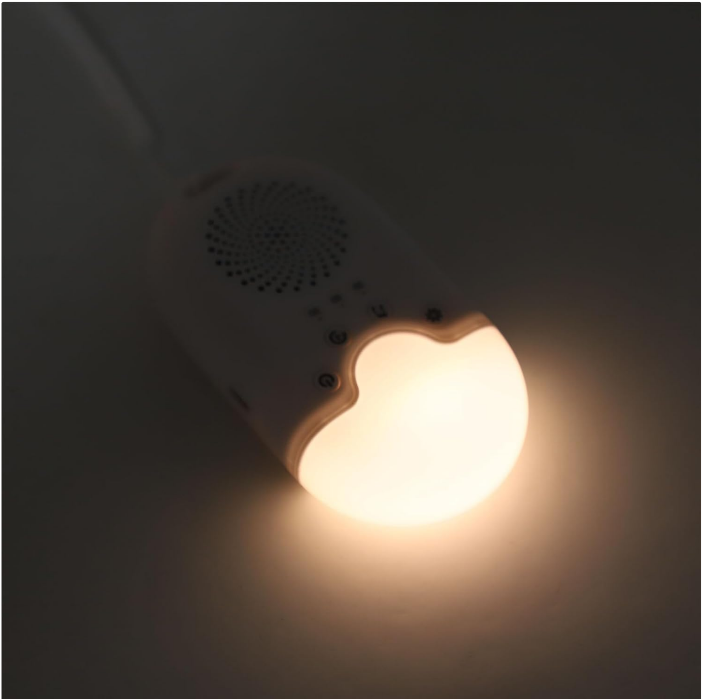
Figure 2: Close-up of the control panel. From left to right, the buttons are: Night Light button (snowflake icon), Sound Selection button (music note icon), Timer button (clock icon) with 30, 60, 90 minute indicators, and Power button (universal power icon).
