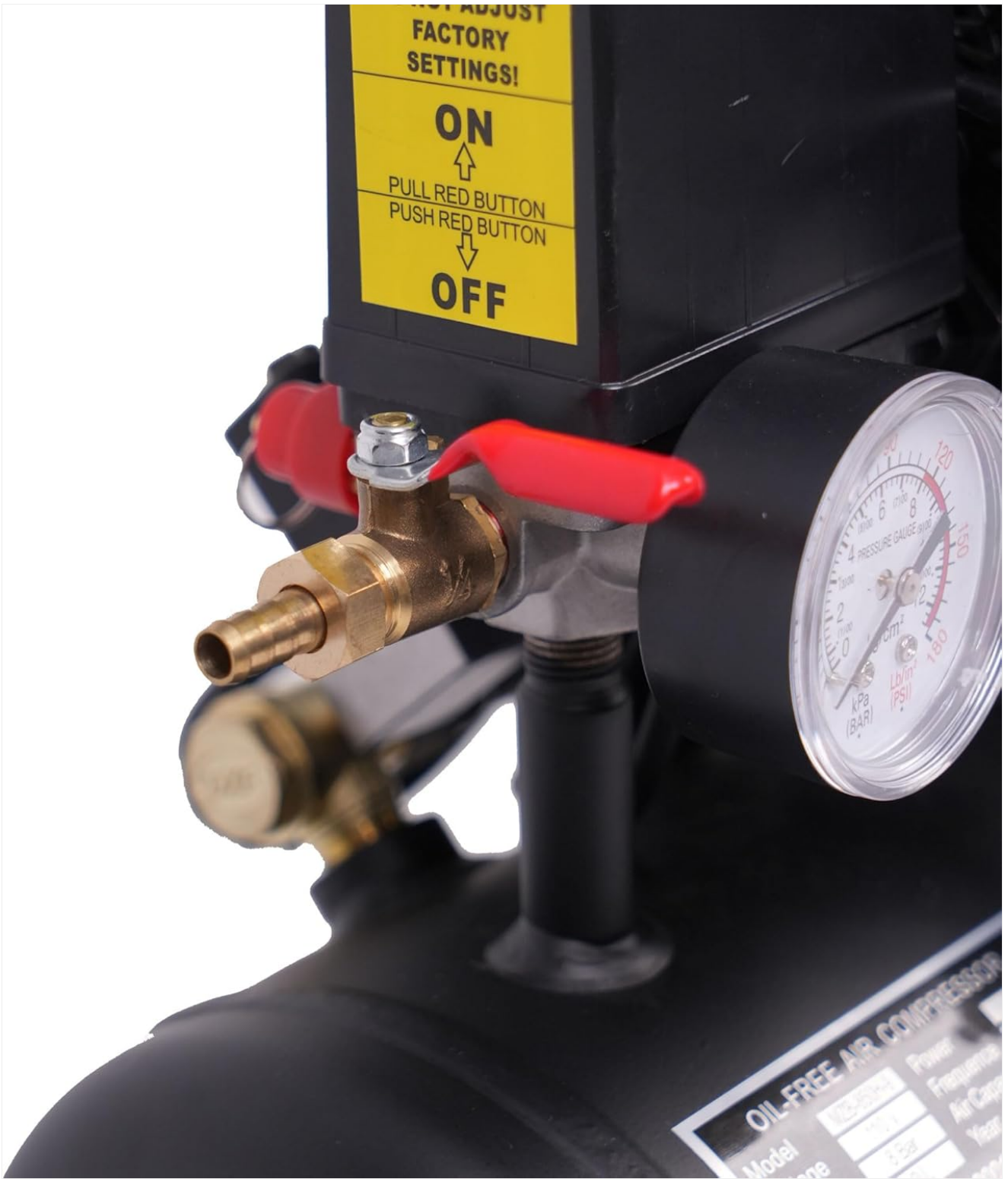
Figure 2.2: Close-up view of the pressure gauge and power control switch.
