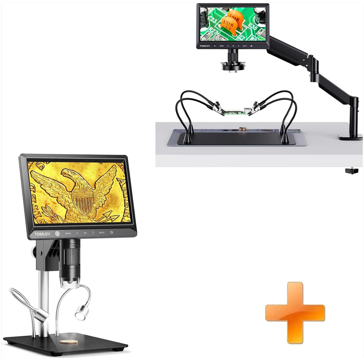
Image: Complete TOMLOV DM702 Flex-S system including the digital microscope, flexible boom arm, and soldering helping hands station.
