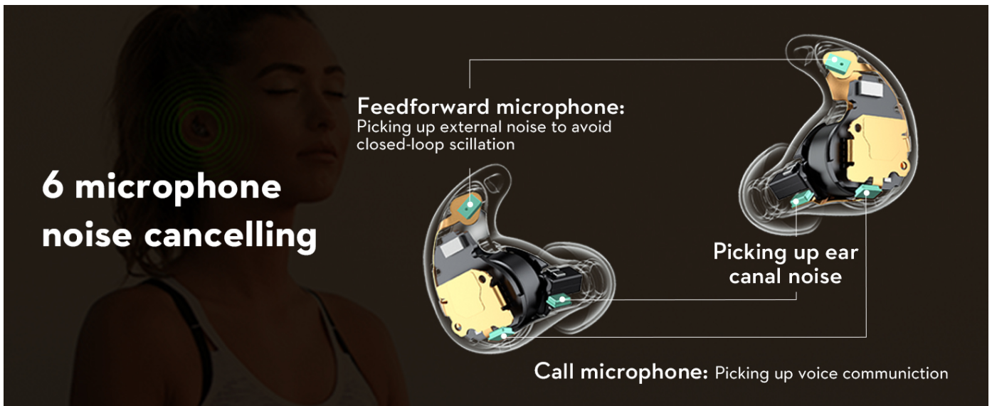
Image: Detailed diagram showing the placement and function of the six microphones for noise cancellation, including feedforward, ear canal, and call microphones.
