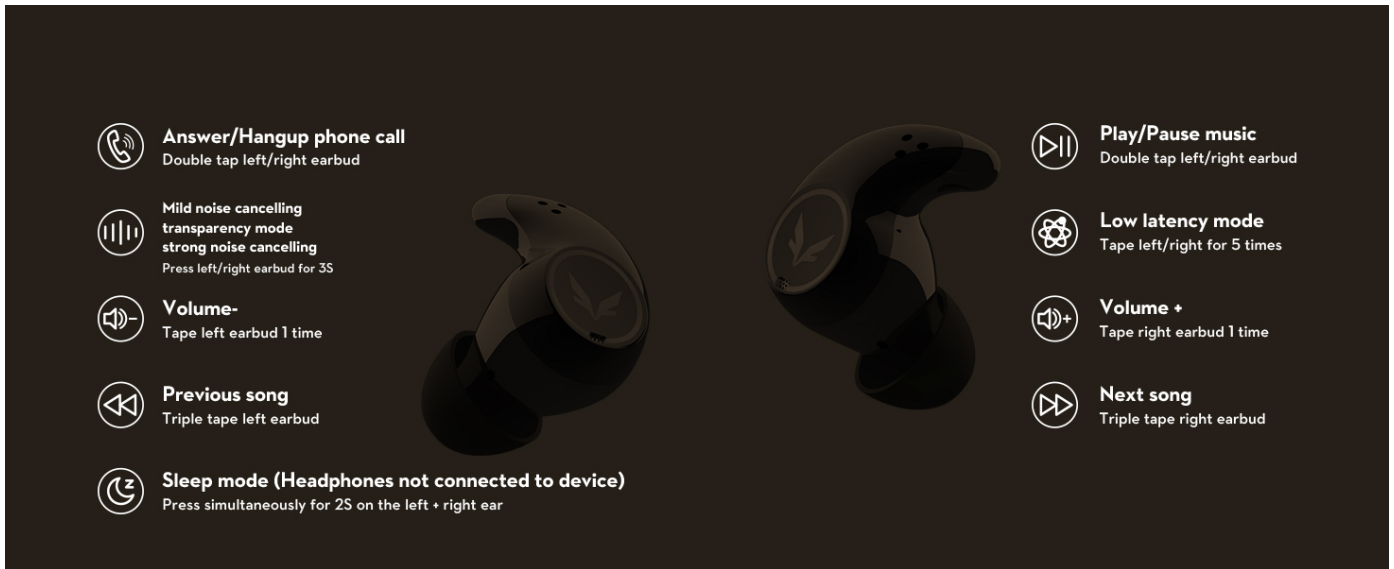
Image: Diagram illustrating touch controls on the left and right earbuds.
