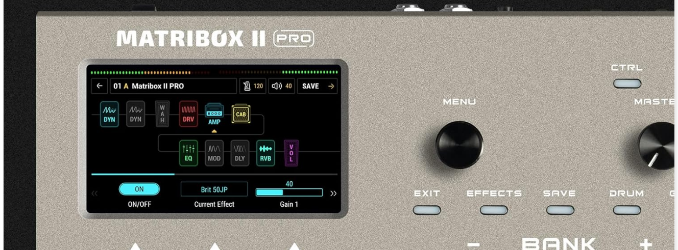
Image 2.2: Visual representation of the effect matrix with various movable effect modules.
