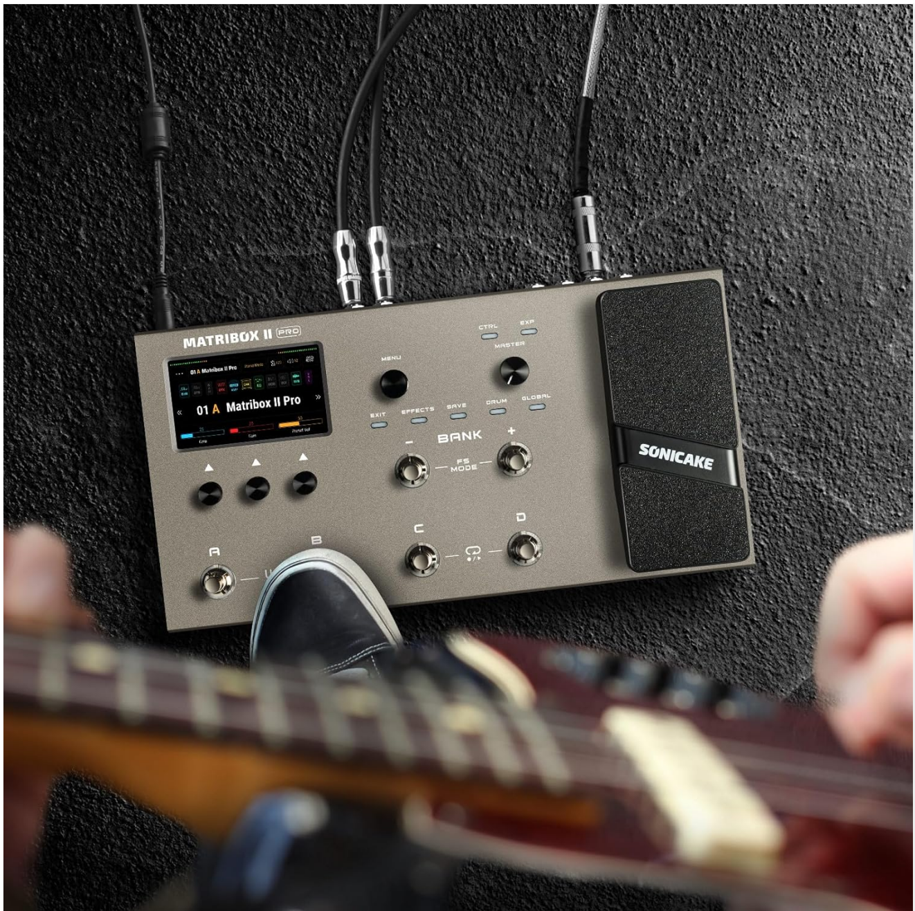
Image 4.1: Overview of the Matribox II Pro's top panel, showing the display, knobs, and footswitches.
