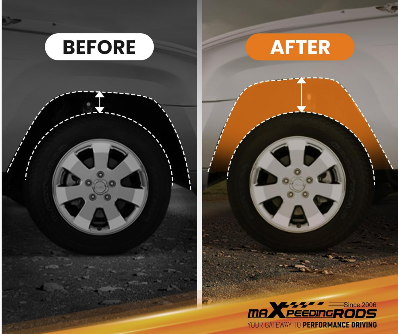
Image 1.1: Visual representation of a vehicle before and after the installation of a 2-inch front and 2-inch rear lift kit, demonstrating increased wheel well clearance.
