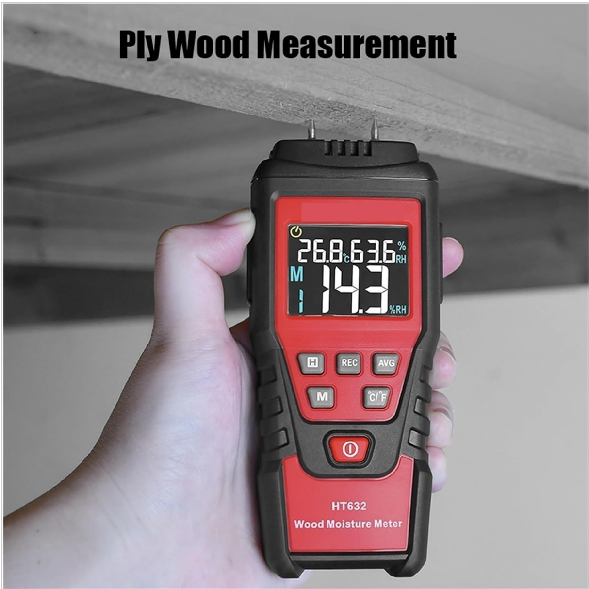
Image 5.1: Measuring moisture content in plywood.
