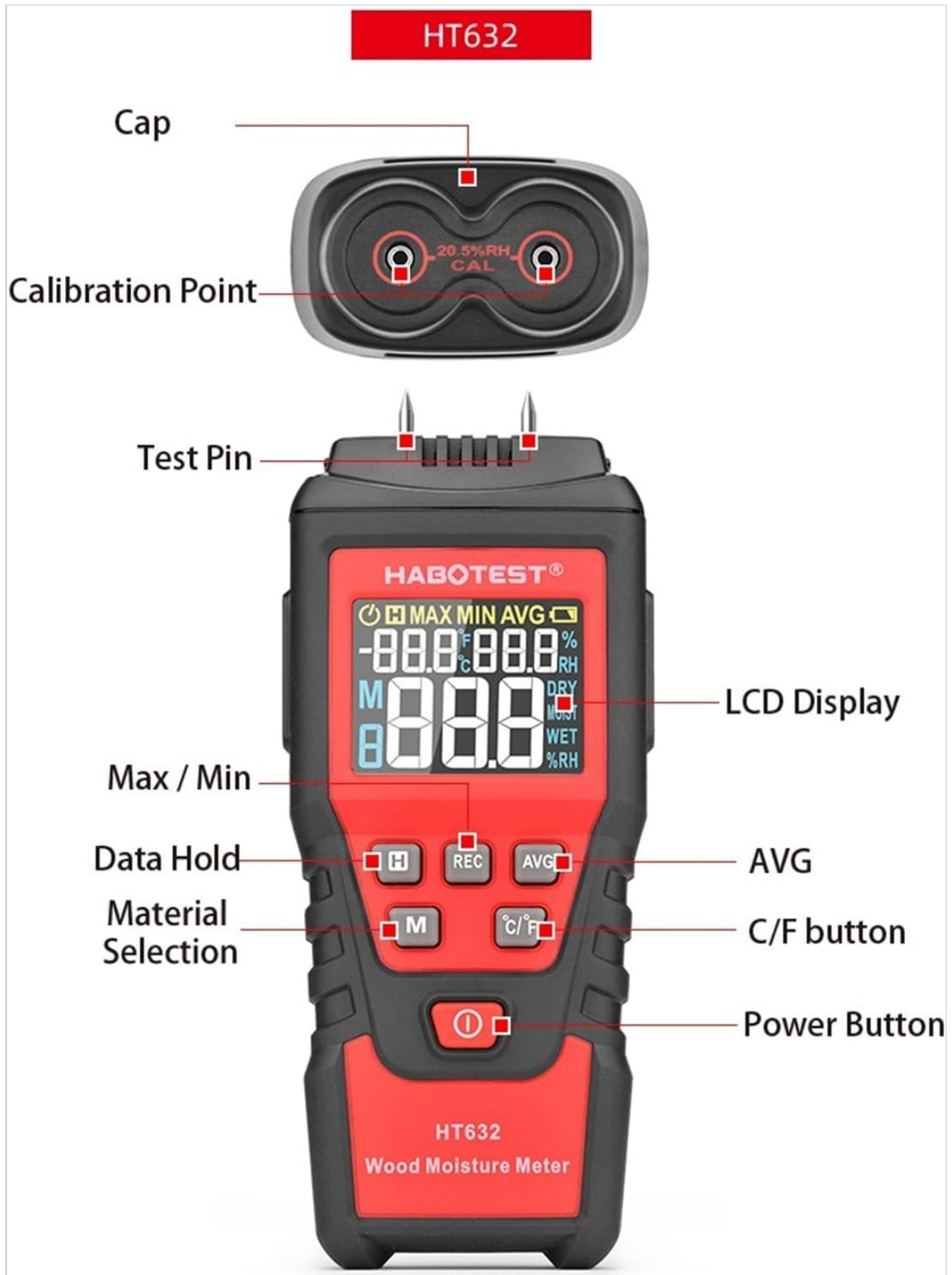
Image 3.1: Labeled components of the HT632 Moisture Meter.
