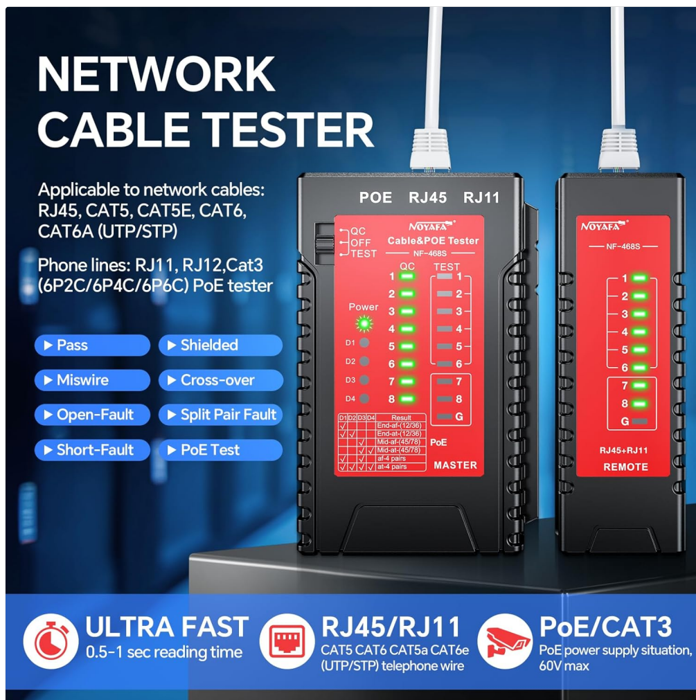
Image: Visual representation of different cable fault indications on the NOYAF NF-468S, including pass, shielded, miswire, cross-over, open-fault, split pair fault, and PoE test results.
