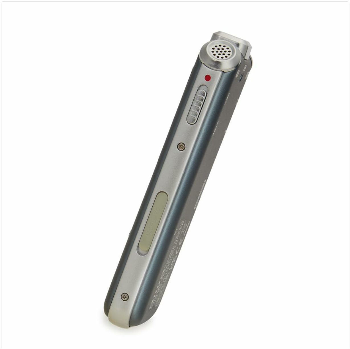
Figure 3: Side view of the recorder, showing the record slider and other side-mounted controls/ports.
